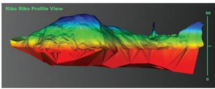
3D model of Riko Riko from combined laser and bathymetric data. Red shows underwater portion. Maximum height is 38.1 meters.
